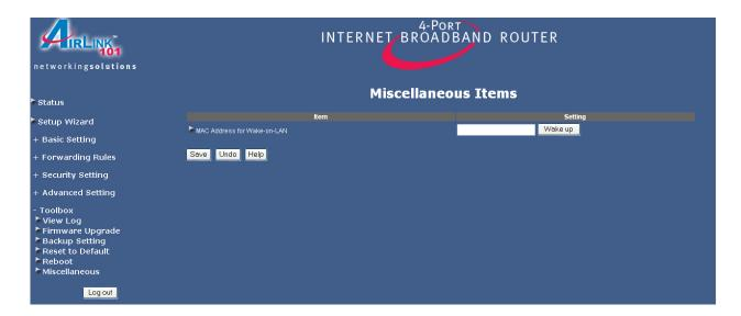
Wake-on-LAN is a technology that enables you to power up a network device remotely. In order to use this feature, the target device must be Wake-on-LAN enabled and you have to know the MAC address of the device, i.e. 00-11-22-33-44-55.
